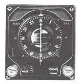
THE COURSE ARROW, COURSE DEVIATION INDICATOR AND HEADING MARKER ARE SLAVED TO THE MAGNETIC HEADING OF THE AIRPLANE (I. E. VERTICAL ON THE FACE OF THE HSI). NO MODE LIGHT IS ILLUMINATED.
