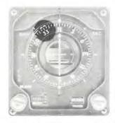
THE HEADING MARKER IS POSITIONED BY THE HEADING SET KNOB TO PROVIDE THE ADI BANK STEERING BAR WITH BANK AND AZIMUTH INFORMATION IN ORDER TO TURN TO THE SELECTED HEADING. THE MAN MODE LIGHT IS ILLUMINATED.
