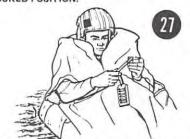
SCREW CARTRIDGE FLARE INTO LAUNCHER WHILE KEEPING FLARE POINTED IN A SAFE DIRECTION.
