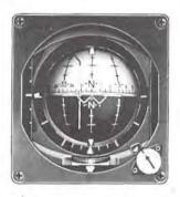
THE BANK STEERING BAR INDICATES -BANK ANGLE STEERING UP TO 30° OF BANK TO APPROACH THE HEADING SELECTED BY THE HEADING SET KNOB ON THE HSI.
