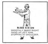
Figure 14-2. Deck/Ground Handling Signals (Sheet 1 of 3)
