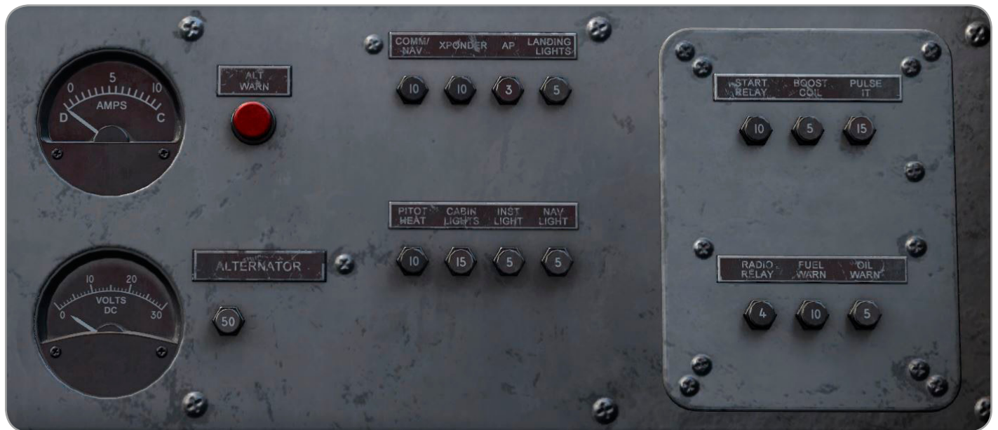
FIGURE 3-7 - ELECTRICAL SYSTEM INDICATORS & CIRCUIT BREAKER PANEL
