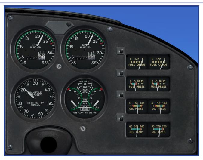
A set of smaller rectangular monitoring gauges are present on the right side of the right hand instrument panel. These gauges are duplicated for the left and right hand engines.
