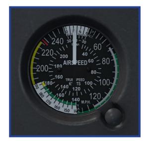
The Twin Comanche features an advanced Airspeed Indicator that includes, in addition to markings in both MPH and Knots, a method for determining True Airspeed (TAS).
