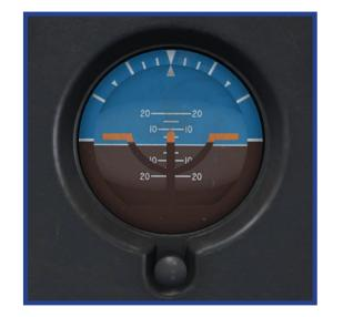
The Artificial Horizon, or Attitude Indicator, informs the pilot of the orientation of the aircraft relative to the horizon. Indicating both pitch (fore and aft tilt) and bank (side to side tilt), it is a primary instrument for flight in instrument meteorological conditions (IMC).
