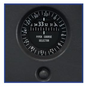
The course selector in the Twin Comanche functions as an useful heading selector and indicator. It consists of a rotating compass card, a vertical lubber line, and a horizontal compass dial.
