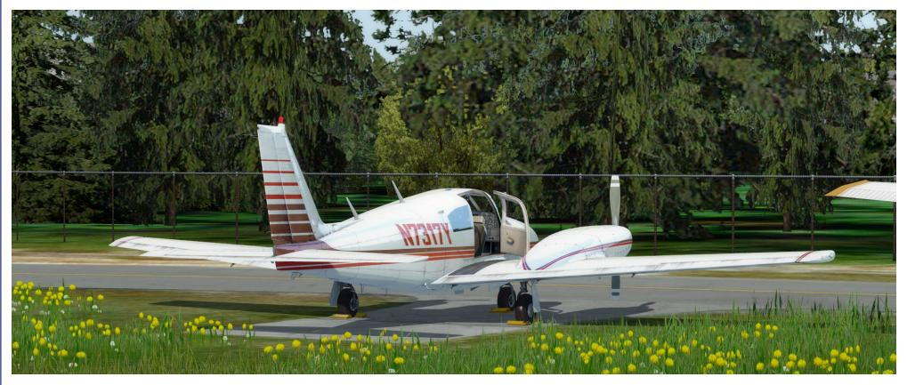
One of the primary reasons for the popularity of the Twin Comanche was its ability to extract decent speed from minimum horsepower and fuel consumption. The fuel injected variant of the extremely popular 0-320 family, the I0-320-B1A, produced 160 horsepower and enabled the PA-30 to cruise at a comfortable 170 knots while burning just 17 gph. With the Time-Between-Overhaul (TBO) listed at 2000 hours, the 0-320 family is highly regarded for both simplicity and durability.
